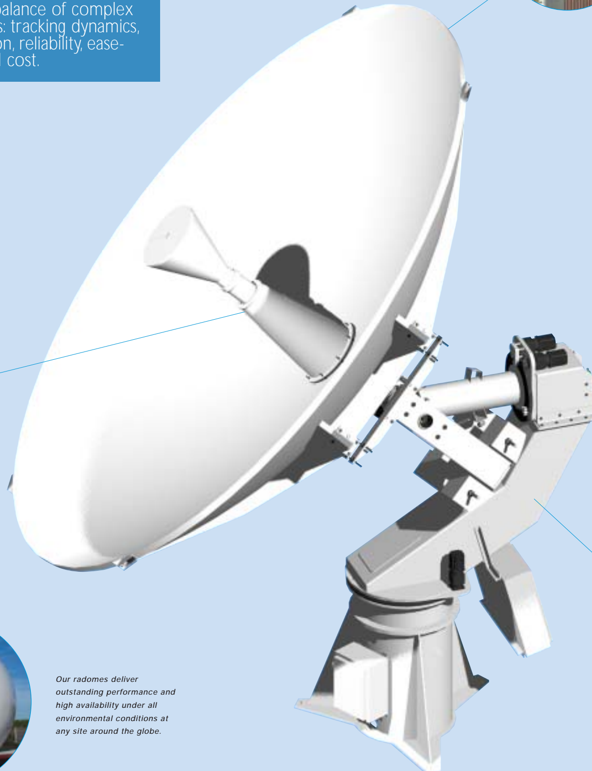
Dual-shaped, carbon composite reflectors in Cassegrain geometry with monopod supports result in high aperture efficiency.
